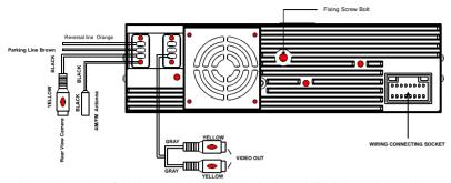
Note: 1. after connecting the Parking Line, the video on the small monitor of the front panel will be display only after braking the car.
